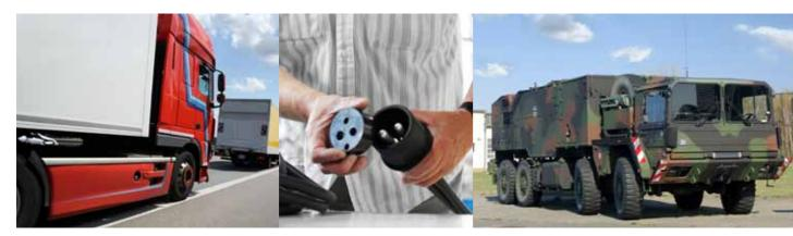
Because of the special requirements, special standards apply for plug connections in vehicle construction. On the one hand, they must be able to withstand a high level of strain, for example due to vibrations or dirt. On the other hand, they are exposed to the effects of weathering, such as heat, cold and damp.
